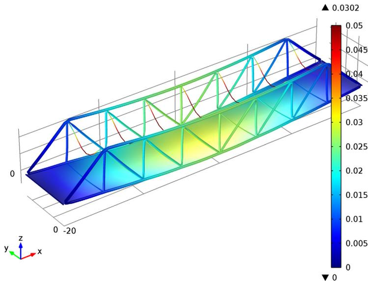
Figure 2: Deformation under self weight.
