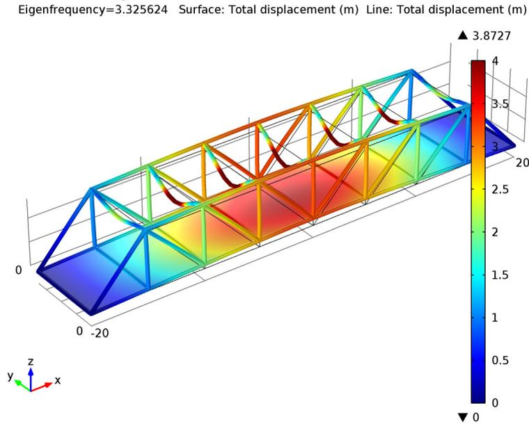
Figure 5: The 9th eigenmode.
