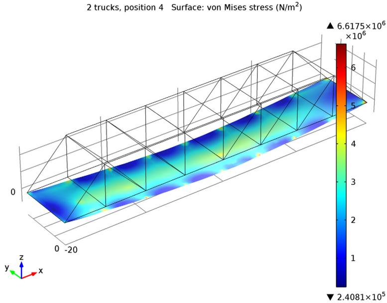
Figure 4: Truck load analysis: Stresses in the bridge deck with two trucks are on the bridge.
