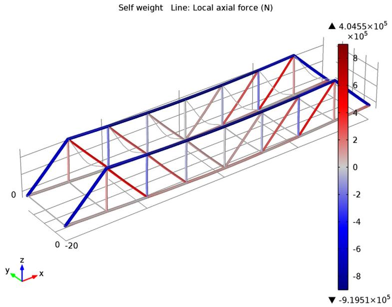
Figure 3: The axial forces in the beams. Red is tension and blue is compression.
