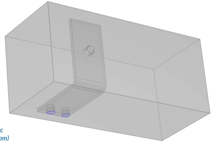
*Geometry selection for the Electric Potential (top) and Ground (bottom) boundary conditions.*
