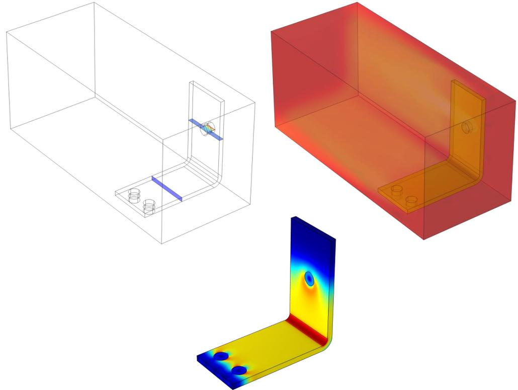
Plots of the results for electric potential (left), temperature (top right), and current density (bottom right).
