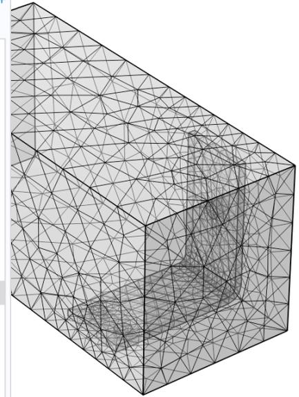
*The meshing sequence and resultant mesh generated for the convective cooling of a busbar tutorial model.*
