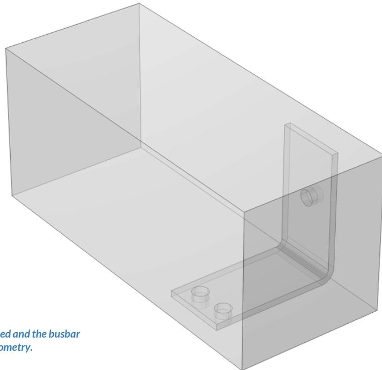
The Import button used and the busbar box tutorial model geometry.
