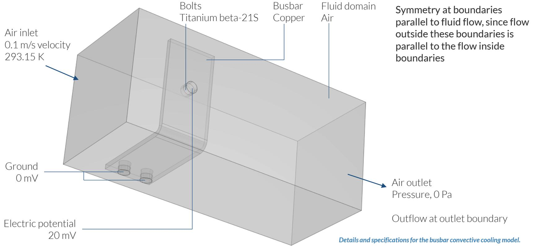
*Details and specifications for the busbar convective cooling model.*
