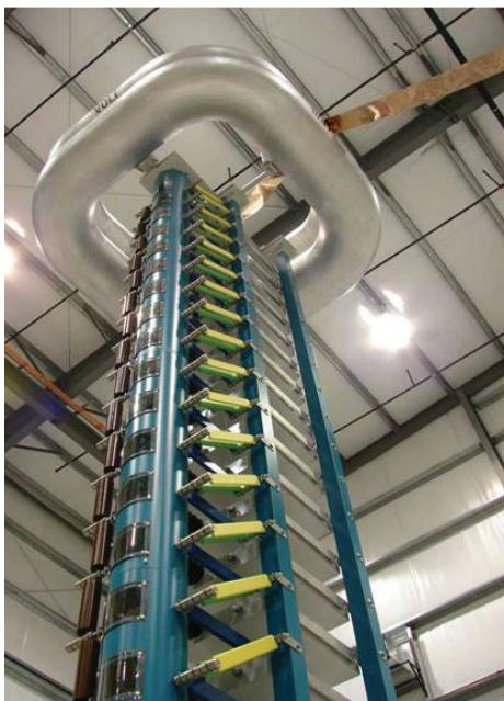
**FIGURE 1.** High-voltage generator (2.4 MV Marx generator) operated by NTS.
