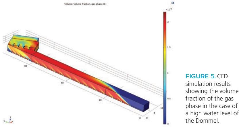
**FIGURE 5.** CFD simulation results showing the volume fraction of the gas phase in the case of a high water level of the Dommel.
