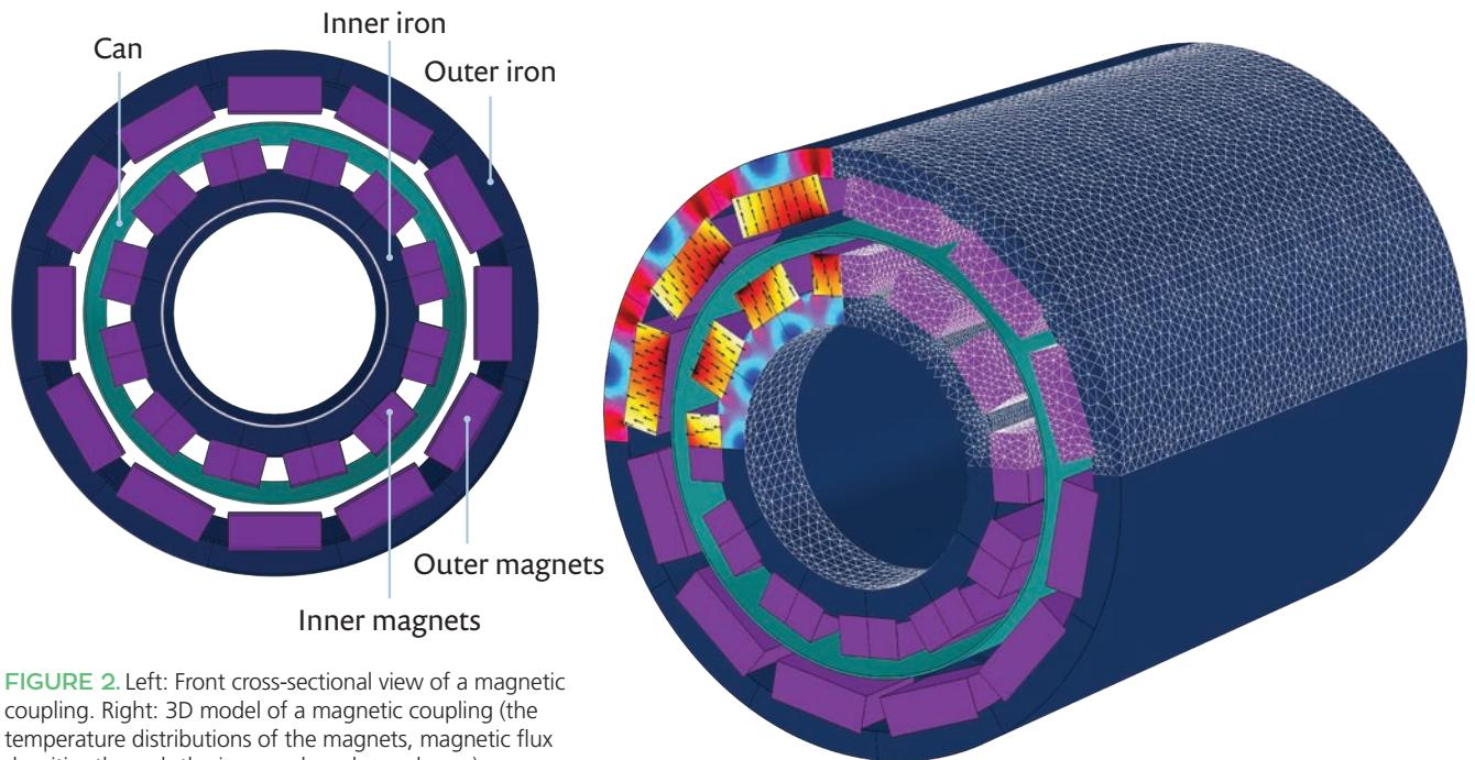
**FIGURE 2.** Left: Front cross-sectional view of a magnetic coupling. Right: 3D model of a magnetic coupling (the temperature distributions of the magnets, magnetic flux densities through the iron, and mesh are shown).
