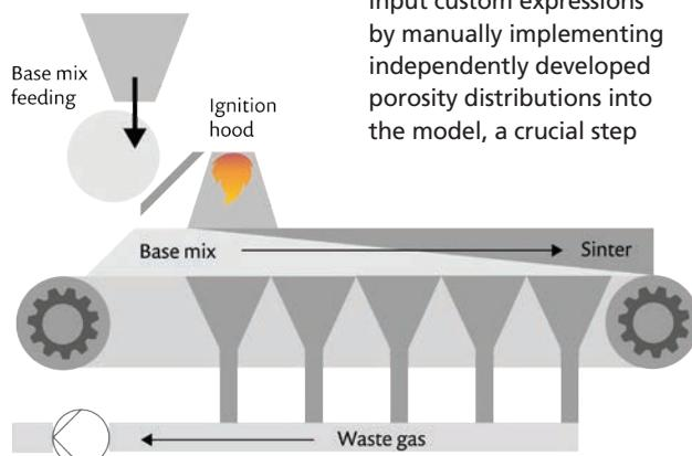
FIGURE 1. Sintering process scheme.
