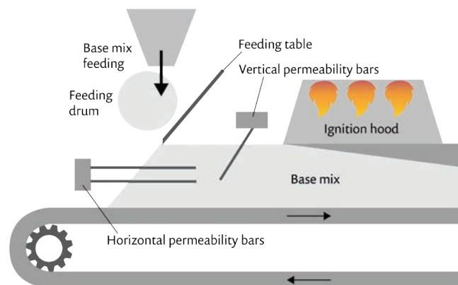
FIGURE 2. Sintering process schematic with permeability bars added.
