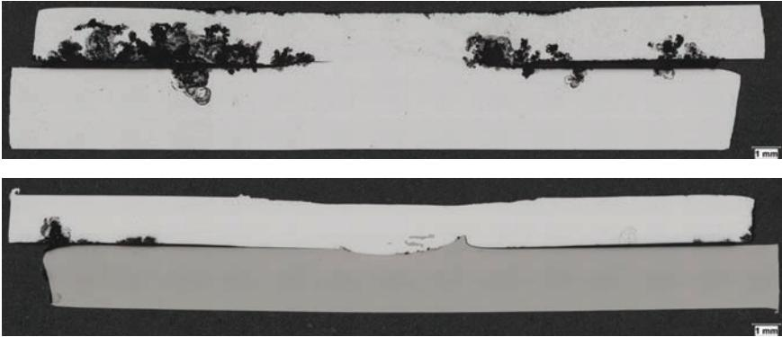
**FIGURE 3.** Cross-sectional view of multimaterial friction-stir welded (FSW) assemblies after a 100,000 km road exposure between a wheel and a mud flap. Top: Dominant crevice mechanism in a AA7000 series to AA6000 series FSW assembly, Bottom: Dominant galvanic corrosion in AA5000 series to stainless steel 300 series FSW assembly.
