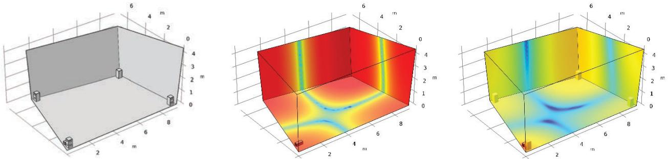
**FIGURE 2.** Left: Geometry of the reverberant chamber with four AER prototypes at the 4 corners. Middle and right: Sound pressure level distribution in the chamber excited on mode 110 at 35.3 Hz without and with absorbers, respectively.
