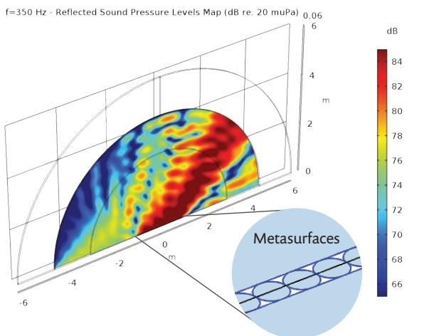
**FIGURE 5.** Reflected sound pressure levels with 32x32 unit cells at  $f = 350$  Hz, for a prescribed reflected angle of  $60^\circ$ .
