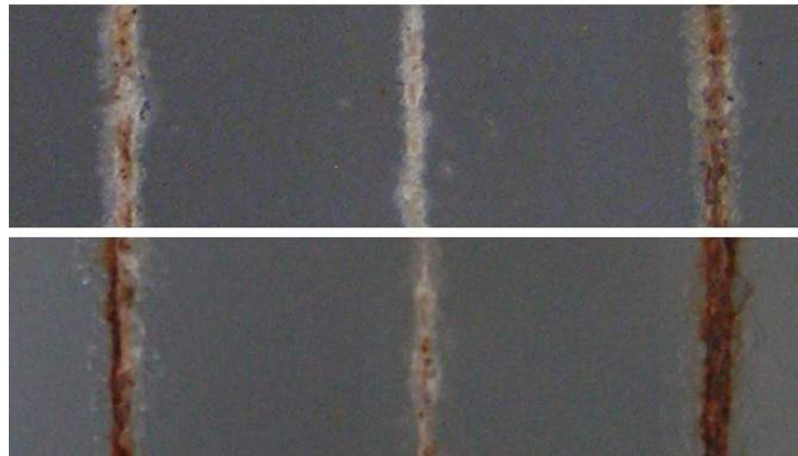
FIGURE 4. A corrosion test on a galvanized steel sheet showing visible corrosion in the scratched layers (view from above). Bösch created several initial scratches of varying depths and widths in order to analyze the influence of the scratch size on the delamination process. Results are shown after one week (top) and five weeks (bottom).
