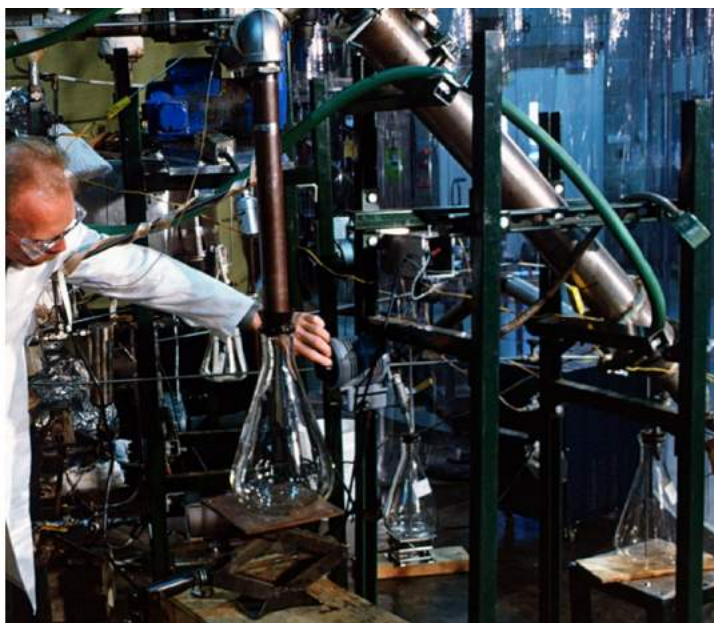
FIGURE 1. In preparation for pyrolysis, the woody biomass shown at left has been milled and may also undergo additional chemical treatment. Several physical processes including heat transfer, mass transfer, chemical reactions, and phase change must be taken into account to develop a complete model of pyrolysis, shown at right. The flask in the photo collects the condensed bio-oil vapors resulting from pyrolysis in a pre-commercial reactor. Photo credits: Warren Gretz, NREL 05756 (left) and Phil Shepherd, NREL 03677 (right).
