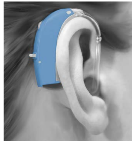
FIGURE 1. A typical BTE hearing aid includes microphones, vibration insulation, and a receiver, among other components. The tight spacing of these components invites troublesome acoustic and mechanical feedback. (Image credit: Knowles Corp.)
