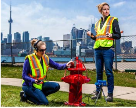
FIGURE 2. The LeakFinderST™ correlator is a compact, intuitive leak noise correlator.
