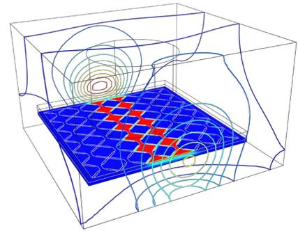
Example design box showing a touch sensor with electric field lines modeled using the AC/DC Module, an add-on product to COMSOL Multiphysics® software.
