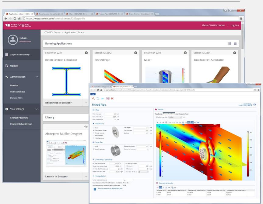
**BRING YOUR SIMULATION TO COLLEAGUES AND CUSTOMERS WITH SIMULATION APPS AND COMSOL SERVER™** Choose which parts of your simulation to share with colleagues, collaborators, and clients. (Image above: COMSOL app of a finned pipe, used to evaluate the thermal performance of various geometries.)
