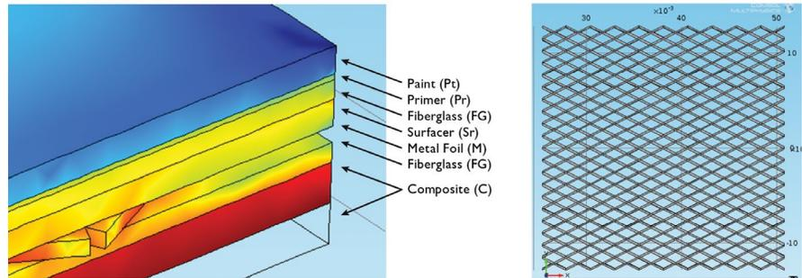
At left is the composite structure layup from the COMSOL Multiphysics® software model and, at right, the geometry of the expanded metal foil. SWD and LWD correspond to short way dimension and long way dimension. The mesh aspect ratio, SWD/LWD, is one of the parameters varied in the study.
