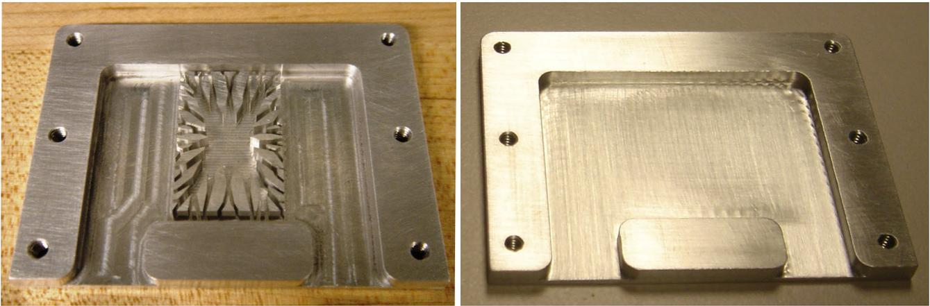
Prototype aluminum cold plates with (left) and without (right) a representative hierarchical microchannel topology.
