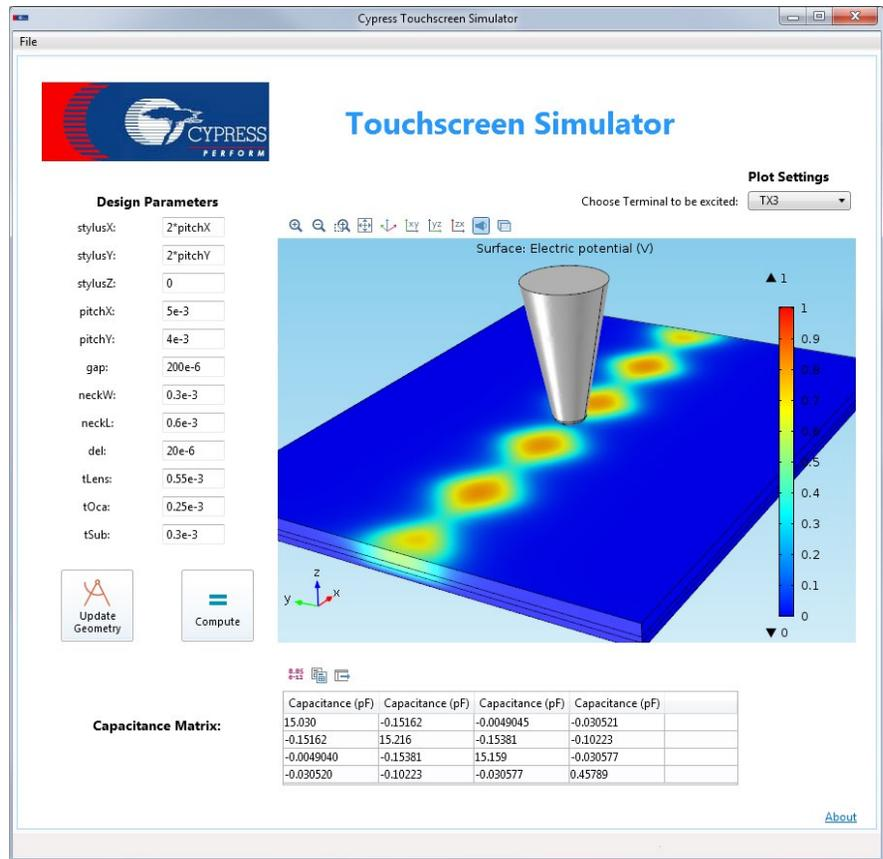
Simulation app based on a COMSOL® software model used to support the design of touch-based capacitive sensors. The app user can change design parameters ranging from the finger location to the thickness of different layers in the sensor. A drop-down list can be used to select a solution corresponding to the excitation of different sensor traces.
